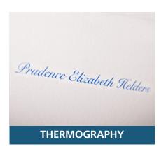
Also known as raised printing, this process simulates the feel of engraving with a high gloss finish.
